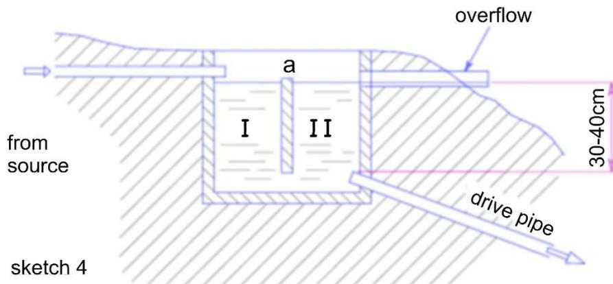
To prevent overflowing of the collection shaft, an overflow facility should be provided (sketches 4 - 6). In the design according to sketch 6, the water not required by the ram can be drained off through the idle plug **b** and through the idle pipe **c**. This design has the advantage that the collection shaft can be emptied and cleaned easily. The overflow must be positioned so that no backflow to the source can occur.
