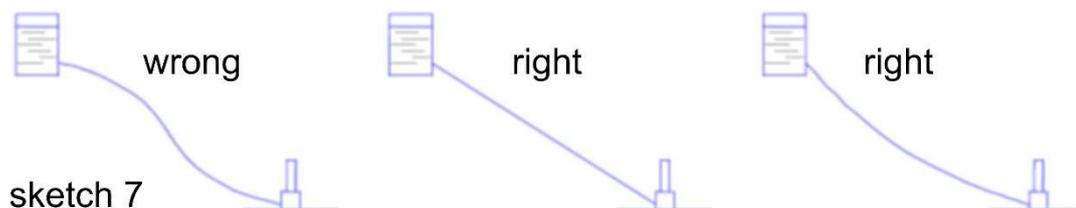
No more than 15° angles may be used, never 45° or even 90° angles. These would severely impair the flow and restrict or even make it impossible for the ram to operate properly.
